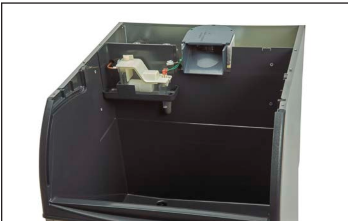
Evaporator Cover Removed
