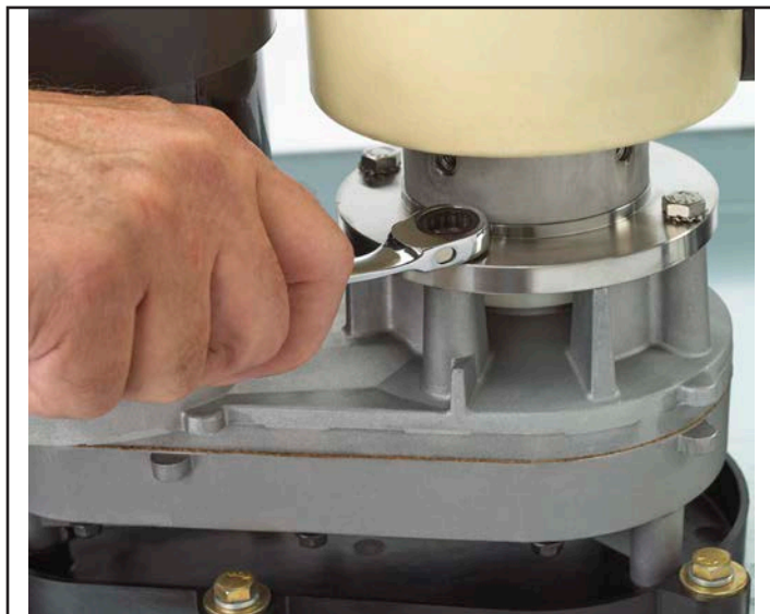
Remove Evaporator Bolts
