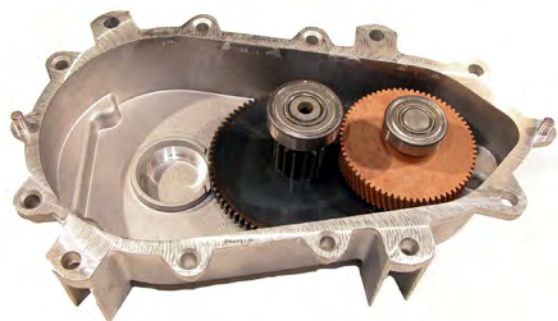
Gear Case with First and Second Gears
