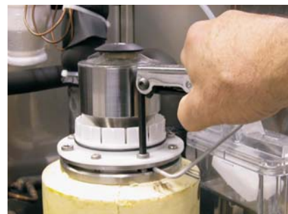
Remove allen head cap screws
