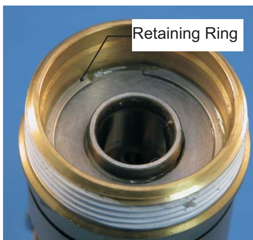
Roller Section Installed
