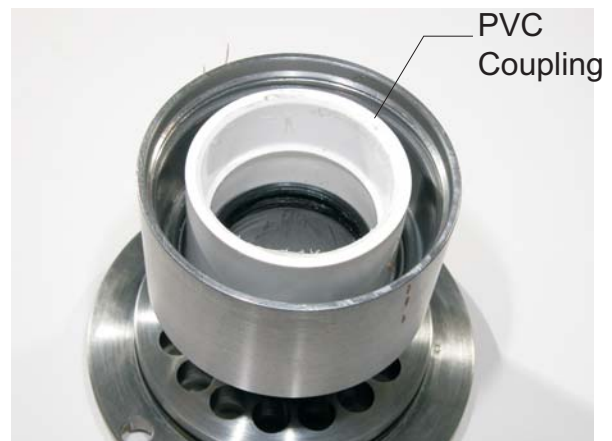
Inserting Lip Seal Using PVC Coupling
