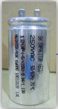
Running Capacitor 250VAC-12 \mu F
