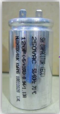
Running Capacitor 250VAC-12 \mu F
