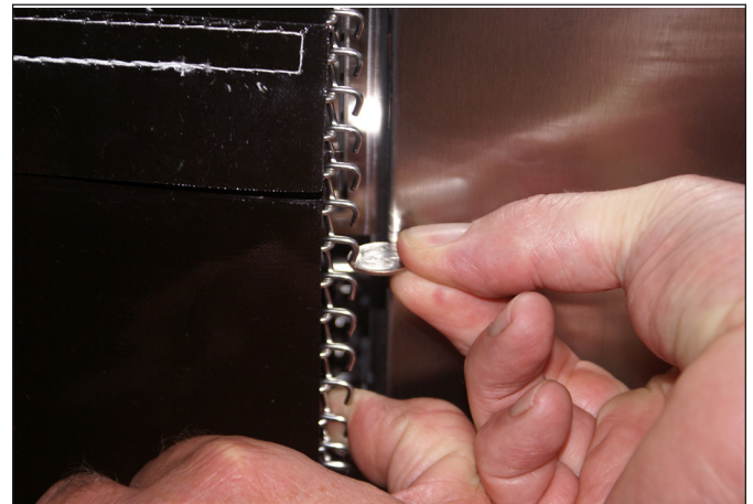
Figure 11. Measuring Conveyor Belt Chain
