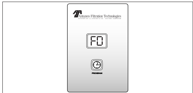
Figure 11. LED Display for Flush Duration
