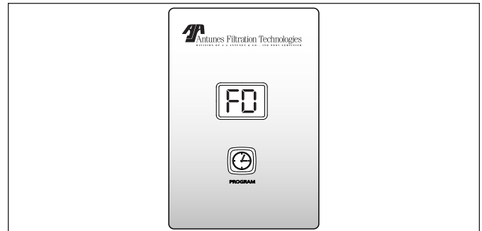
Figure 7. LED Display for Flush Duration Mode
