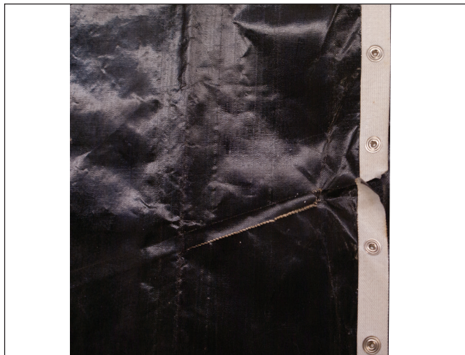
BELT IS MISSING SNAPS AND IS DAMAGED. REPLACE BELT.
