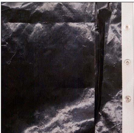
Belt is torn and folded. Replace all Belts.
