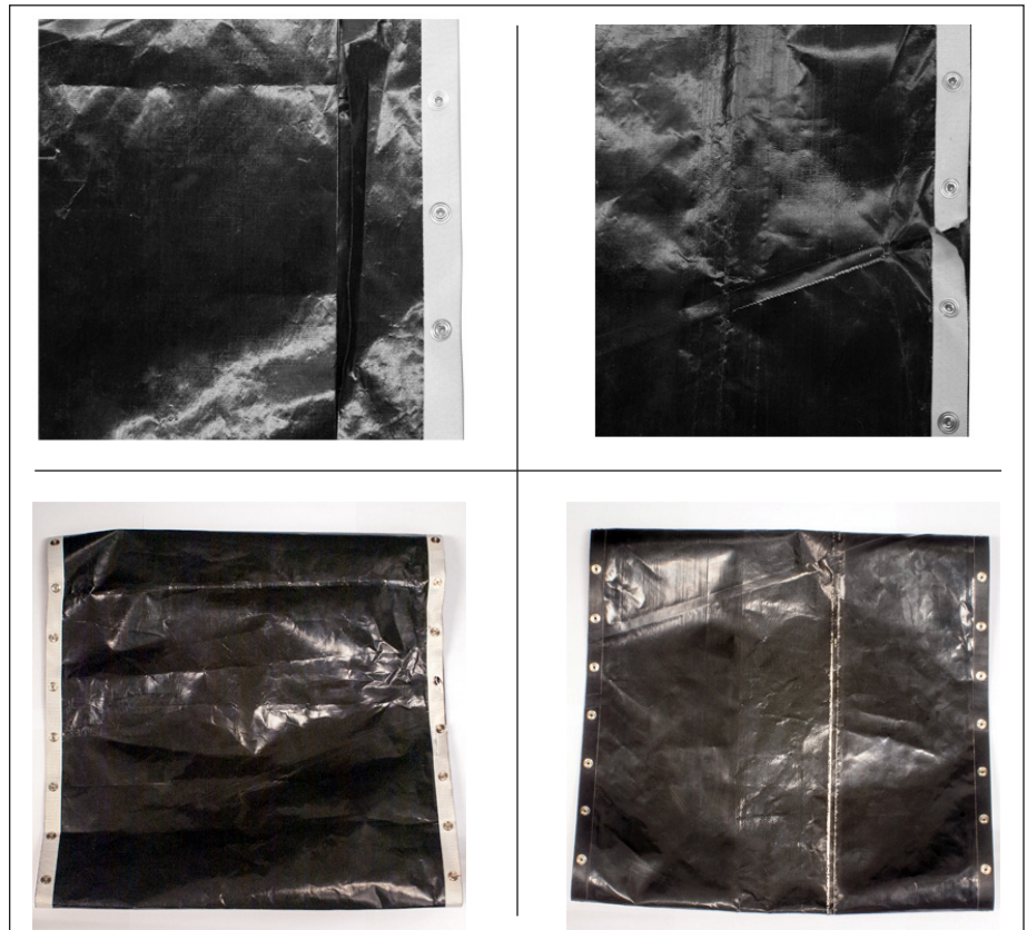
Figure 6. - Examples of Damaged Belt Wraps
