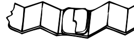
Figure 16B - As turbulator strip is installed in the tube, interlock the sections.
