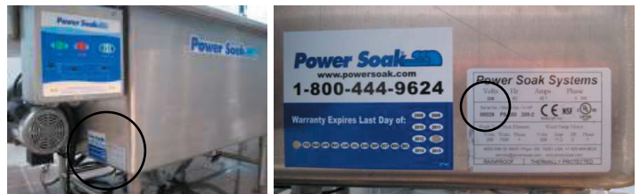
The serial number is 5-6 digits long and located on the lower corner of the wash tank closest to the controller.
