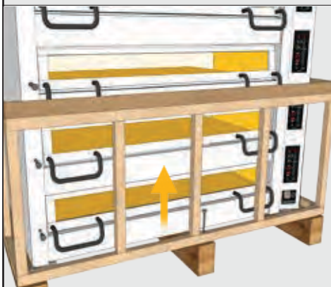
22. Remove the hex bolts and take out the wood cage
