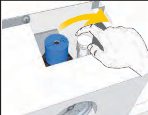
4. Open the Air Relief Valve
