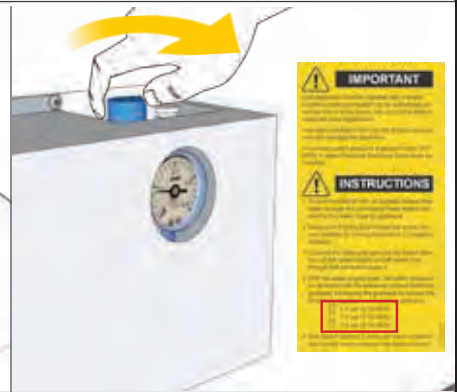
6. Set the water to the pressure marked on the label by turning slowly the Blue Knob regulator in the (+) positive direction. * Repeat for all decks
