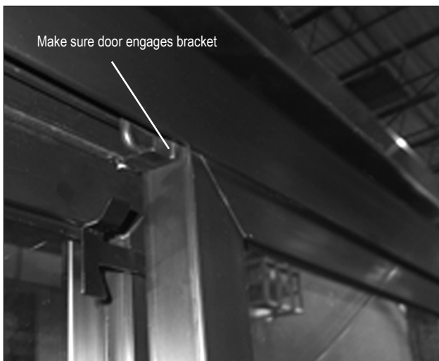
Figure 14: Removing/Installing Sliding Door
