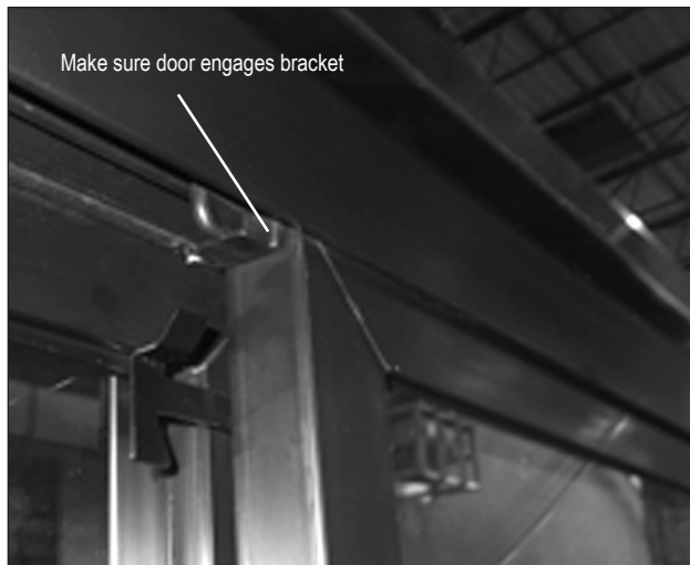
Figure 14: Removing/Installing Sliding Door
