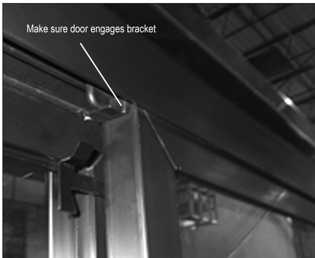
Figure 14: Removing/Installing Sliding Door
