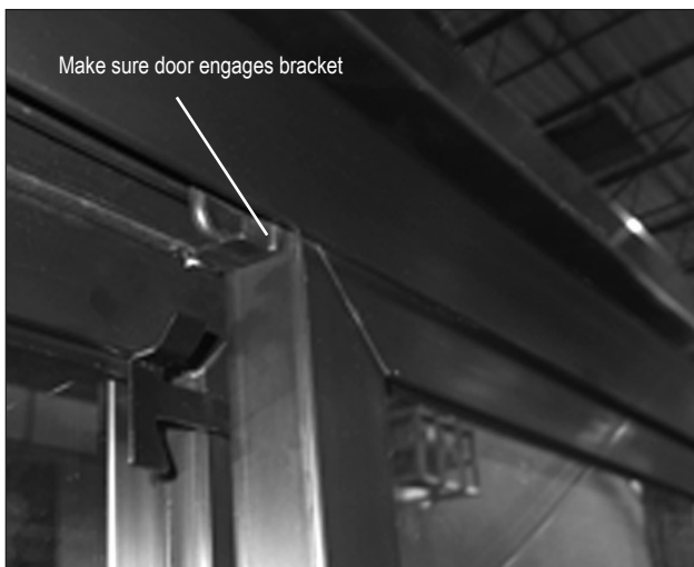
Figure 14: Removing/Installing Sliding Door
