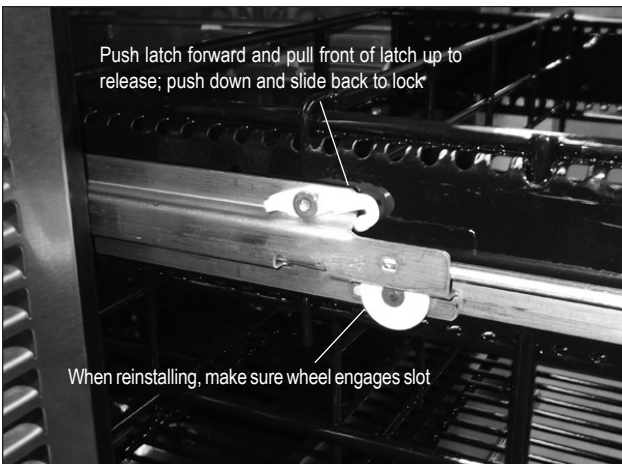
Figure 15. Removing/Installing Drawer
