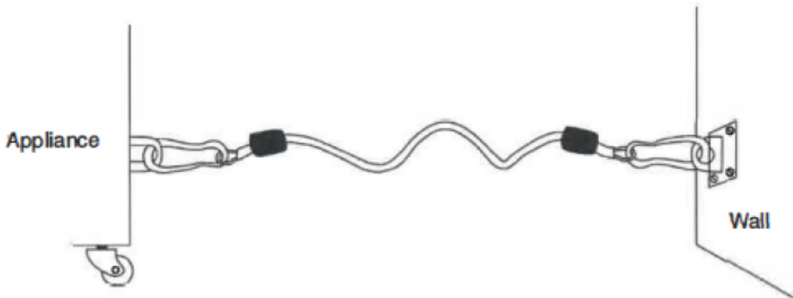
IMPORTANT: This Restraining Device should be ordered with every connector for Movable appliances.
