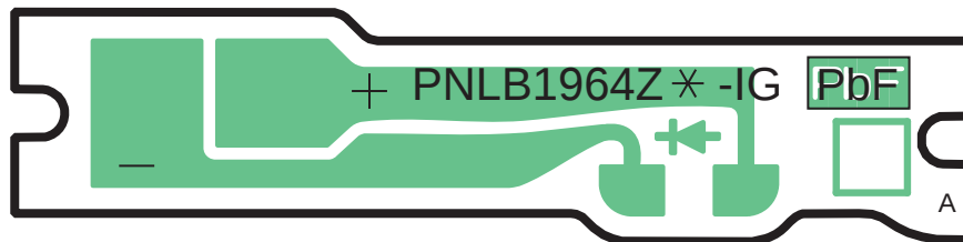
KX-TG6841/6842/6843/6844/6845/6873 CIRCUIT BOARD (Handset_LED (Component View))
