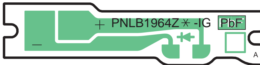
KX-TGA470 CIRCUIT BOARD (Handset_LED (Component View))
