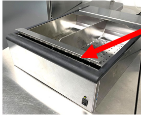
Incorrect placement of the food tray. Front edge is too high.
