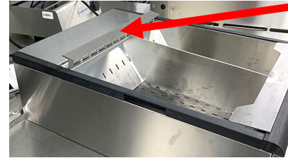
Incorrect placement of the food tray. Food tray is rotated 180°.
