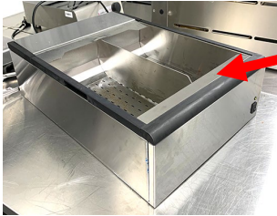
Correct placement of the food tray.
