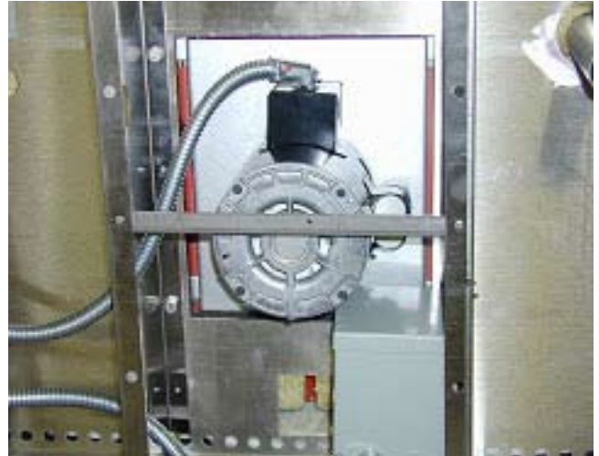
FIG. 40 Support Brace Angle
