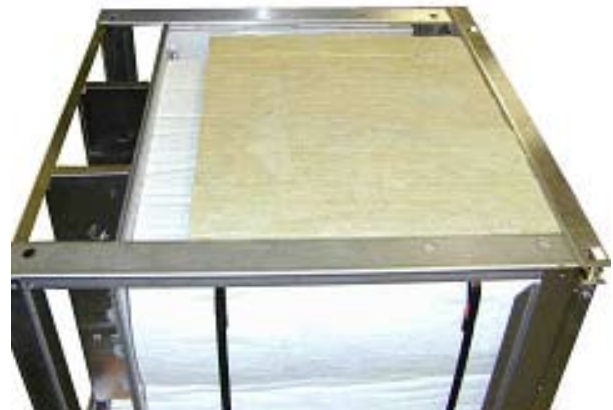
FIG. 24 Top Cavity Insulation
