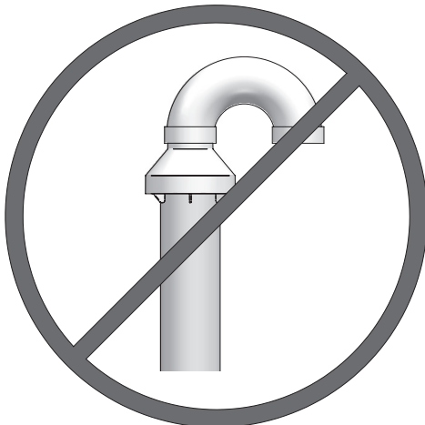
Figure 5-5 Do Not Install U-Bend to Rain Cap
