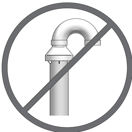
Figure 4-5 Do Not Install U-Bent to Rain Cap
