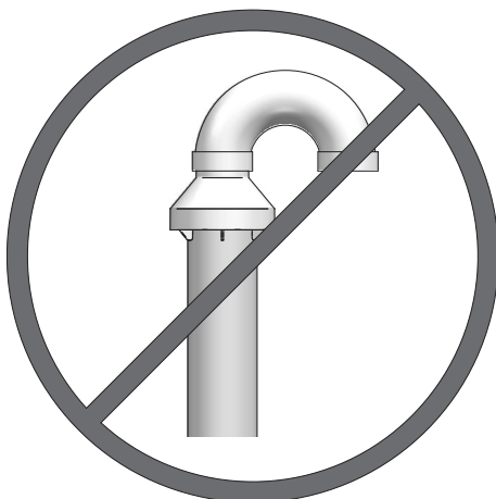
Figure 4-5 Do Not Install U-Bent to Rain Cap
