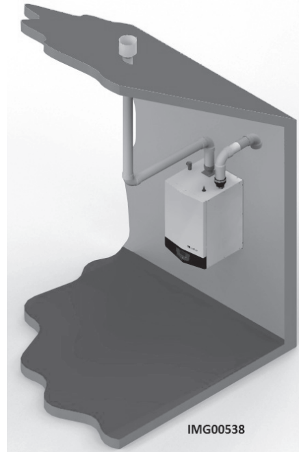
Figure 3-5 Vertical Vent, Sidewall Air
