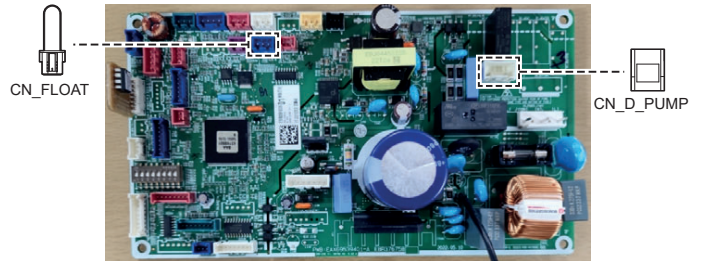
Figure 23: Vertical Installation Conversion Kit PCB Connections (Appearances May Vary).
