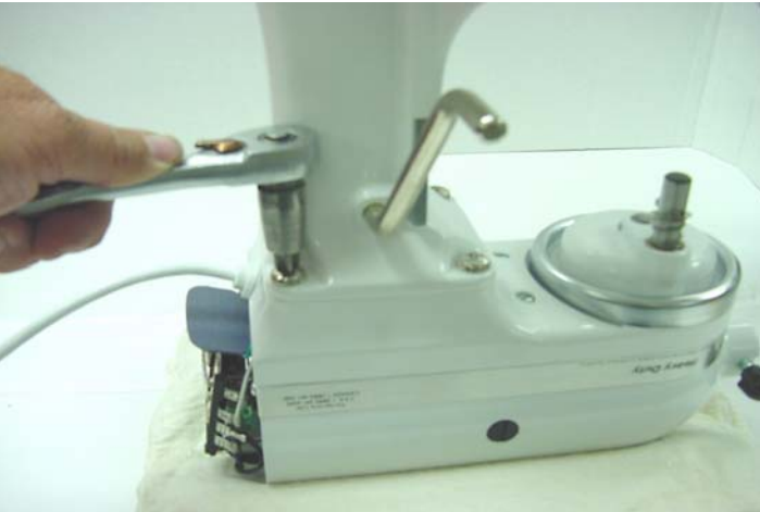
Fig. 84 Four round Phillips head screws must be removed to replace the bowl support assembly.
