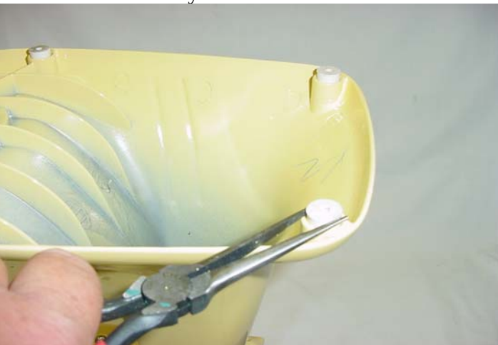
Fig. 71 The pedestal feet should be replaced on older mixers.
