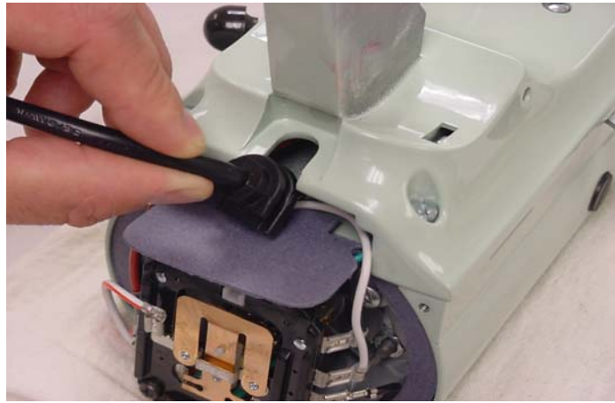
Fig. 8 Pull back on the molded strain relief to remove the power cord from the slot in the bottom cover.
