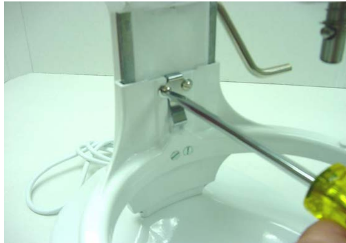
Fig. 95 Two #10-24 x 1/4" screws hold the bowl spring latch in place.
