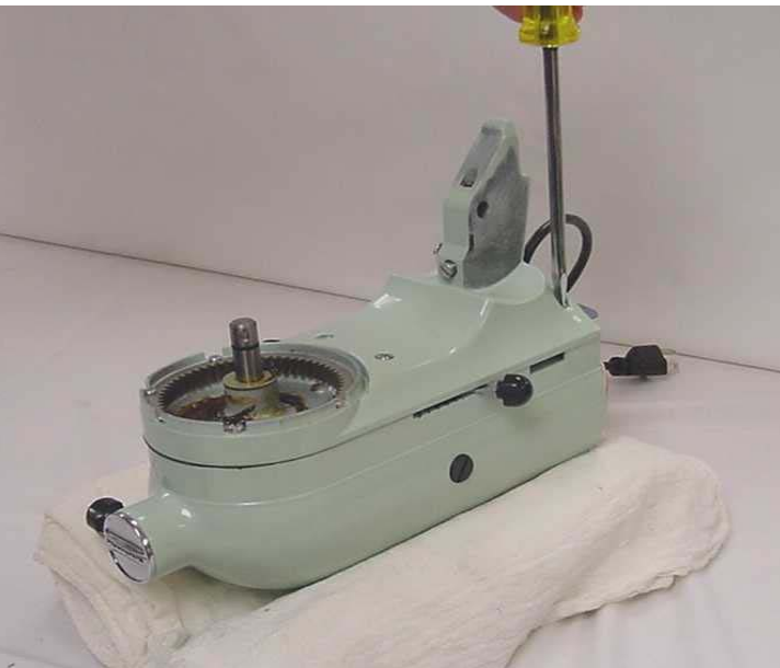
Fig. 11 The bottom cover is removed after removing the four #10-24 filister head screws.
