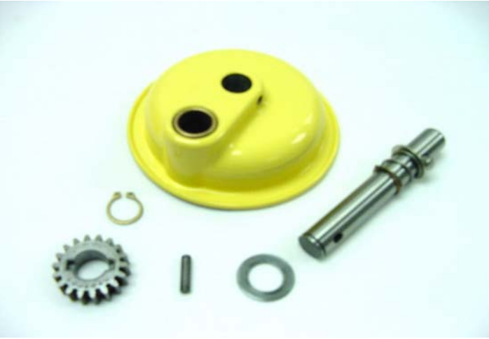
Fig. 66 The planetary components are shown disassembled.
