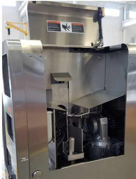
Figure 66. Hopper with Side Access Panel Removed
