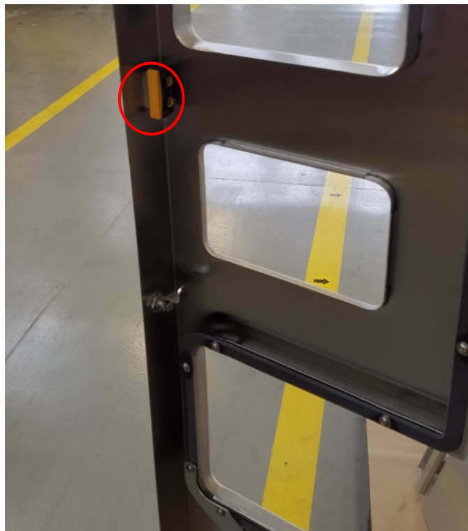
Figure 65. Location of Front Door Safety Magnet
