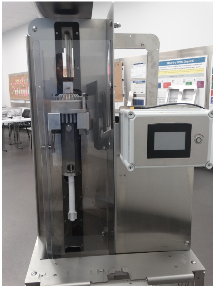
Figure 11. Juicer with All Covers Removed
