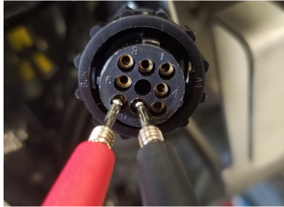
Figure 73. Multimeter Leads, Sockets 8 and 9
