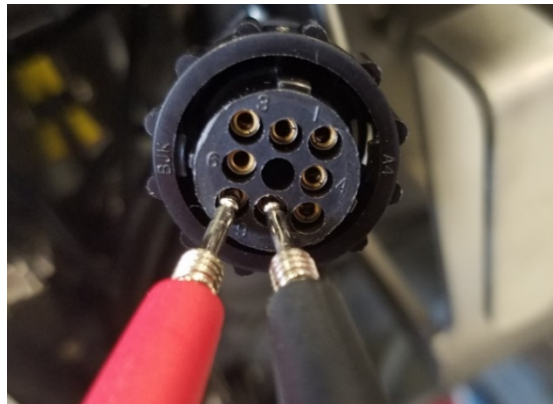
Figure 77. Multimeter Leads, Sockets 8 and 9
