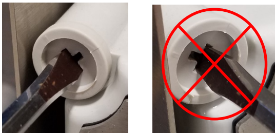
Figure 78. Opening Main Electrical Box
