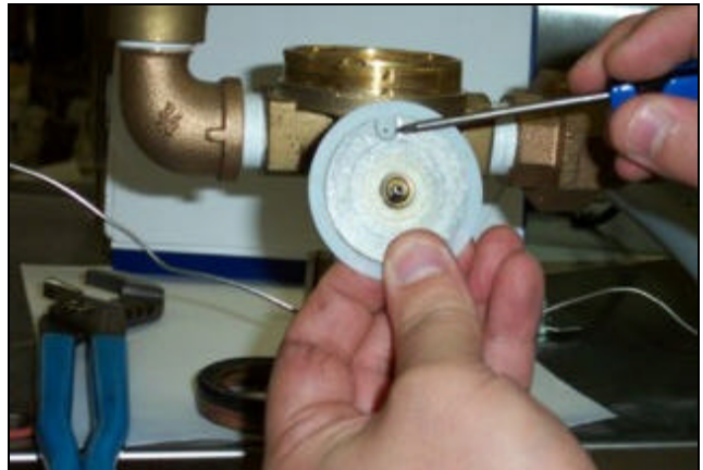
Pointing out the extension hole
