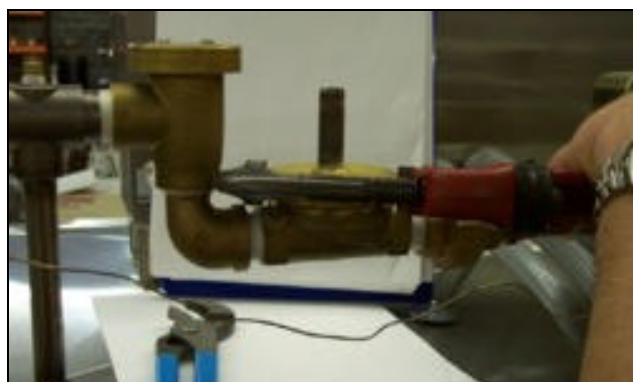
Loosening the valve bonnet
