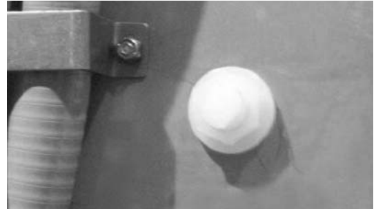
Detergent Connection Point (Machine rear view)
