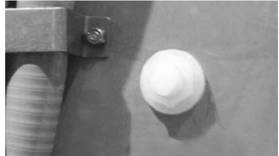
Detergent Connection Point (Machine rear view)
