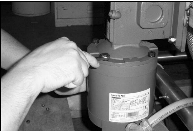
Removing the bolts holding the drive motor to the gear reducer.
