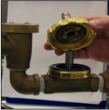
Removing the valve bonnet
