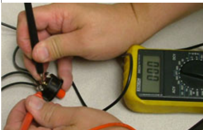
Figure 24. Testing Overload Protector
