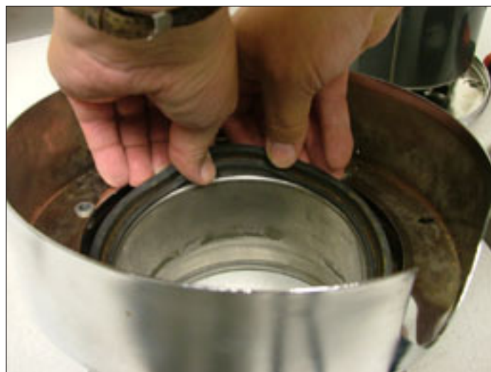
Figure 11. Replacing Shredder Gasket
