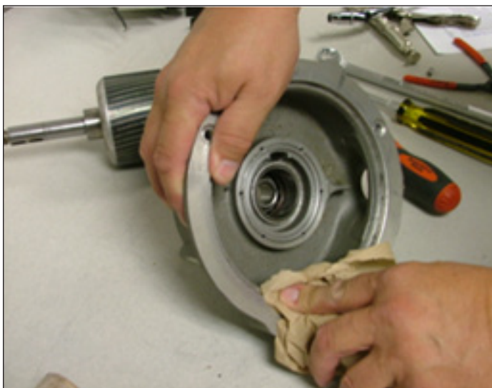
Figure 21. Cleaning Upper End Bell
