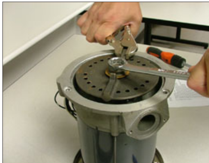
Figure 14. Rotating Shredder Nut
