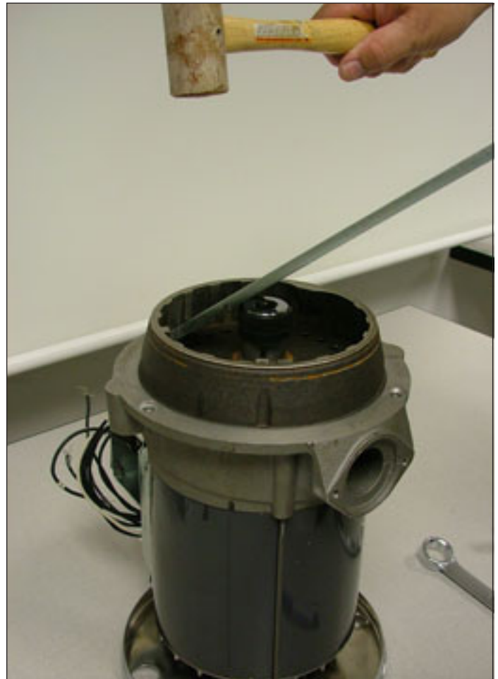
Figure 12. Removing Stationary Shredder
