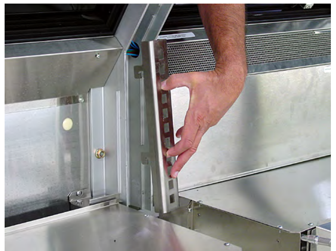
STEP 10 – Lift out lower shelf supports.
