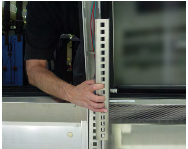
STEP 9 – Lift out upper shelf supports.
