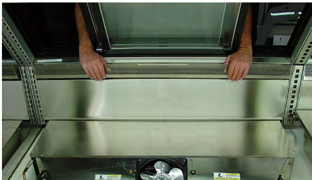
STEP 7 – Lift out discharge air grille.
