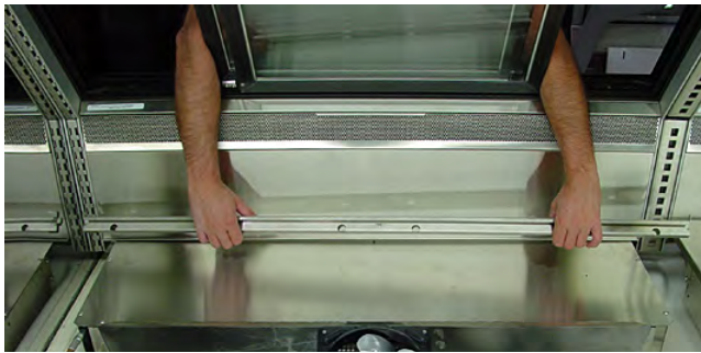
STEP 6 – Lift out display pan support.
