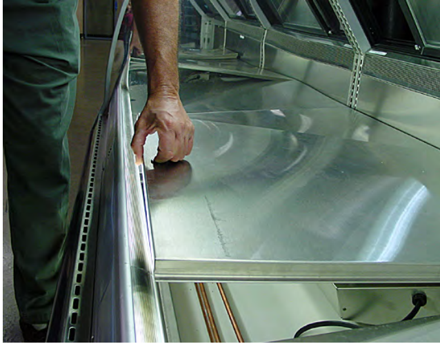
STEP 6 – Lift out display pan support.
