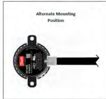
Alternative mounting if downward is not possible. Cable can exit 90 degrees from right or left side. Any angle from downward 0 degrees up to 90 degrees can be used.
