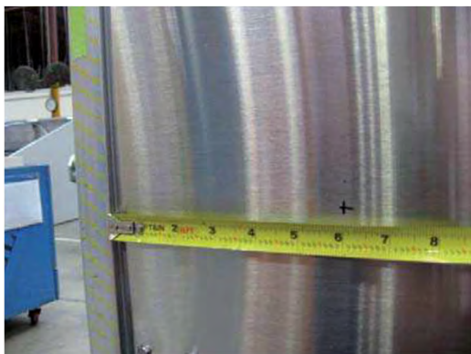
Step 1: Measure 6 inches from wrapping board end.
