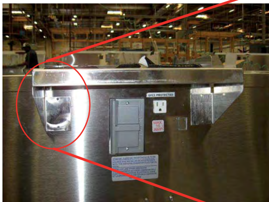
2.- Drill holes and screw in place (with screws provided – Hex Tek S/S
