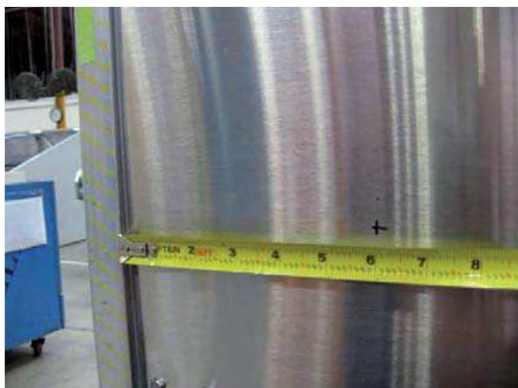
Step 1: Measure 6 inches from wrapping board end.
