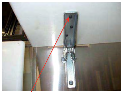
Step 8: Screw bracket into wrap board (screws provided -#8 X 1 1/4")
