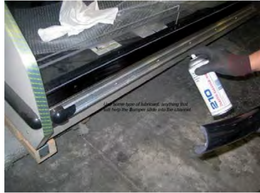
Step 2: Use silicone lubricant to help the bumper slide into the channel.
