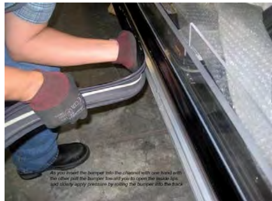
Step 4: As you insert the bumper into the channel with one hand, pull the bumper toward you with the other to open the inside lips. Slowly apply pressure by rolling the bumper into the track. Boston Series 2000
