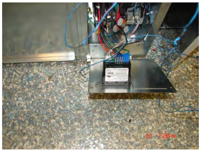
Step 1: Removal of cover: With power off remove screws and pull cover off
