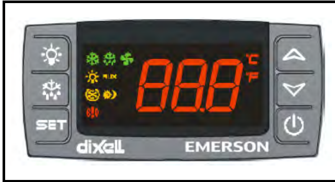
Figure 4-1 - XR75CX Front Panel
