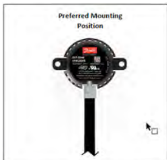
Mount Sensor with cable facing downward if possible. This is to minimize Water ingress from the cable and connector.
