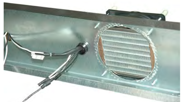
E. Attach heater/fan assembly to fan plenum.
