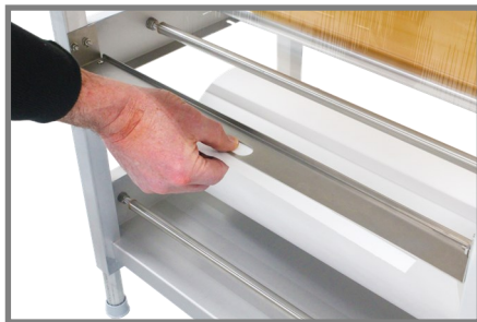
Use the slot-hole on the cutter to grab the threaded butcher paper
