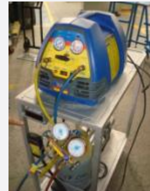
REFRIGERANT RECOVERY MACHINE
